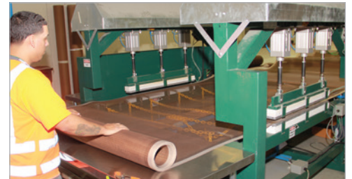
PTFE / Glass fabric edges are heat-sealed on a mesh dryer belt.
